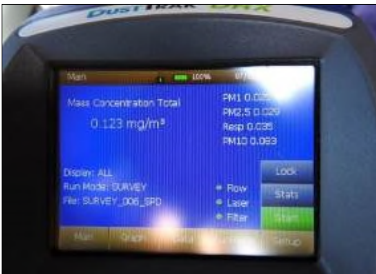
Figure 32: DustTrak DRX dust analyzer
